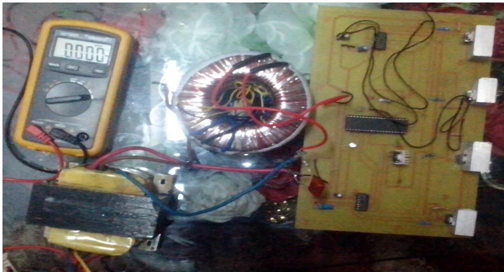
Figure 19: Sine wave Inverter
