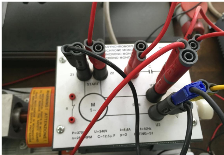
Figure 4:1 Permanent Capacitor Starter Connection Motor
