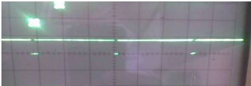
Fig.6.1 The output waveform of the astable multivibrator
