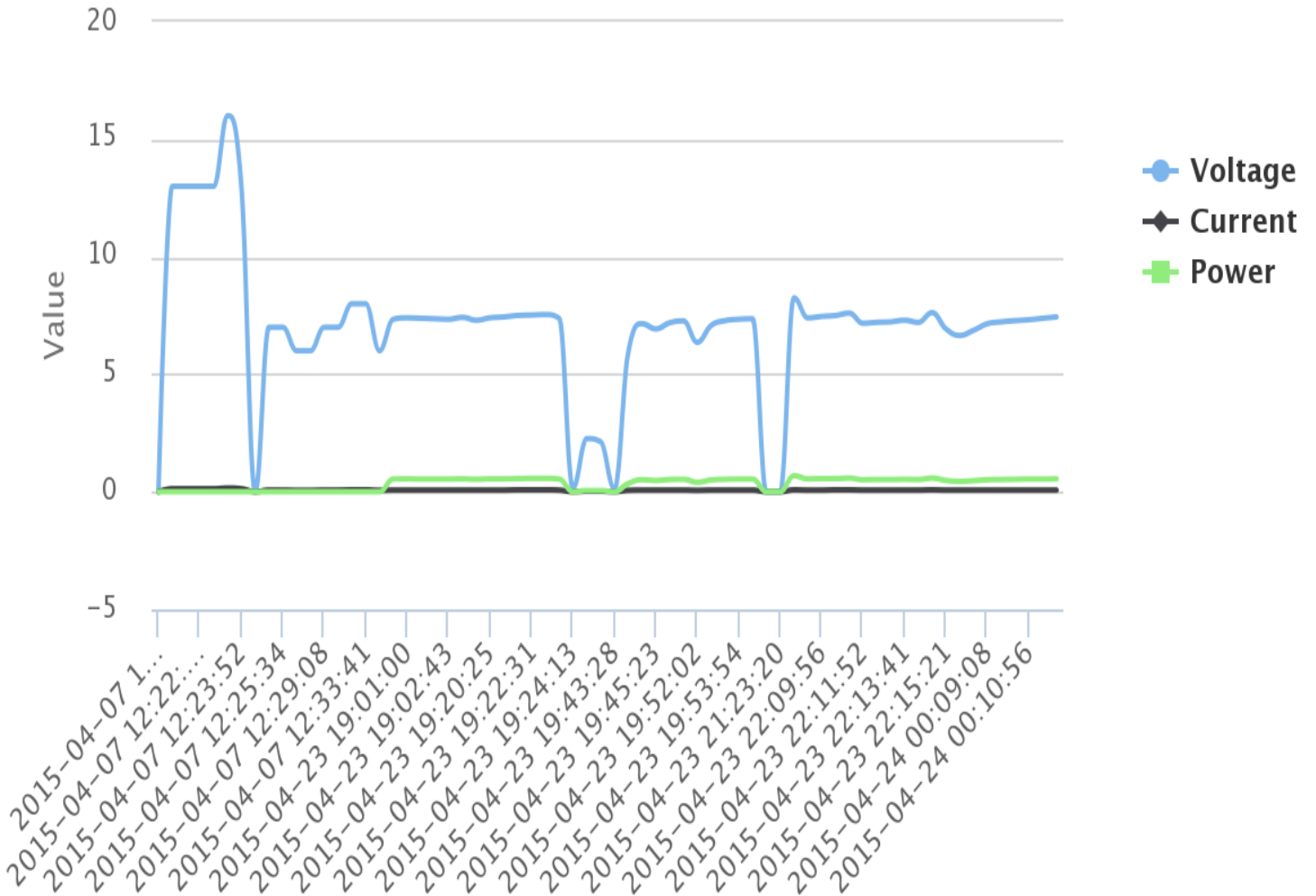
Fig 4.6: A graph of voltage vs current vs power outputs from a 20Watt solar panel under low light conditions.
